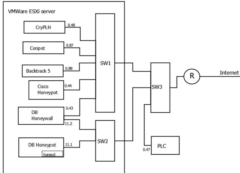
**Fig. 1.** The laboratory setup of the honeypot testbed
