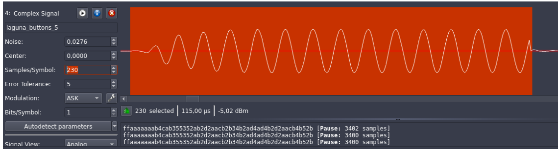
Figure 6.8: Finding out the signal parameters in URH
