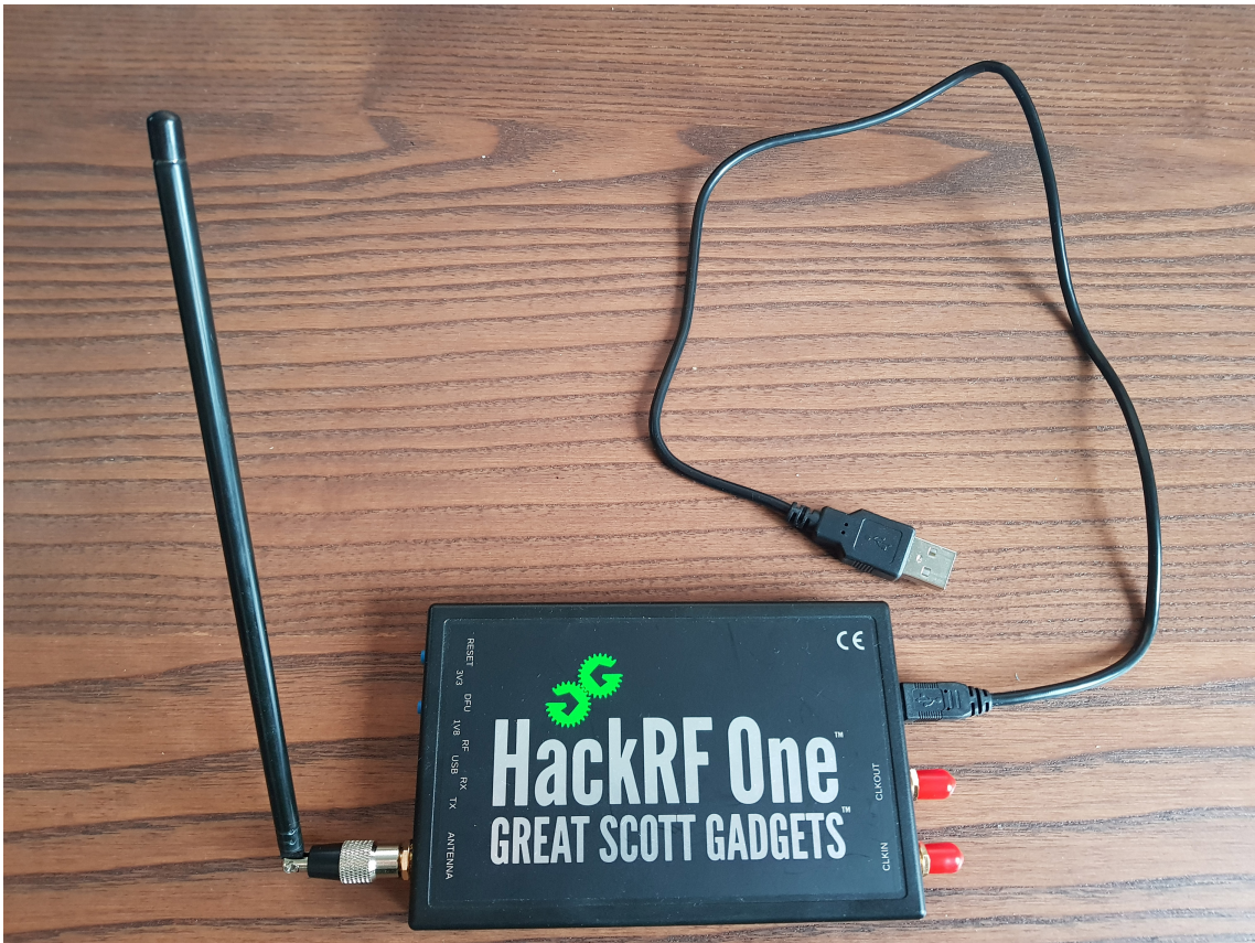
Figure 4.3: The HackRF One hardware device
