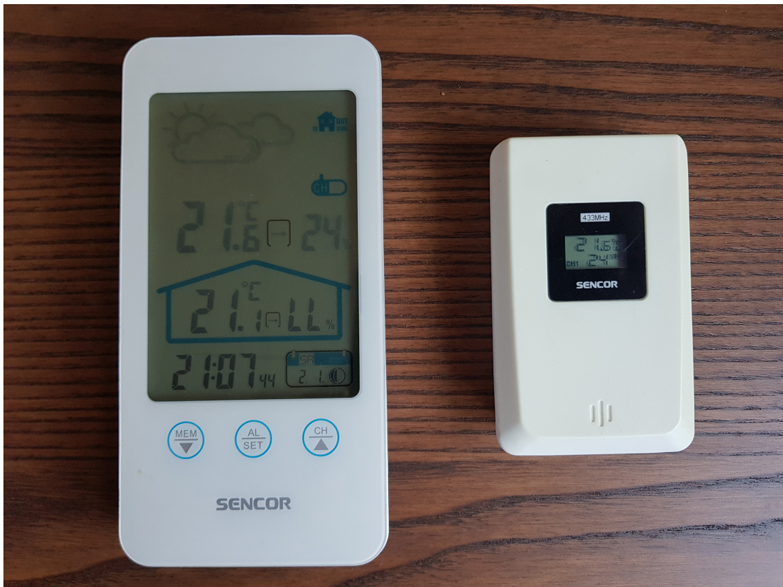
Figure 6.12: Sencor station on the left and the sensor on the right
